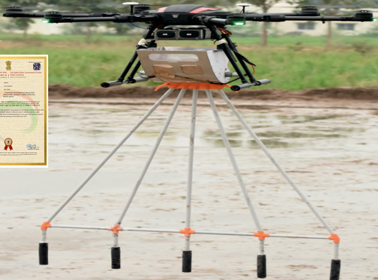
▲ Rice seeding device ( wet direct seeding) attachment to Drone
