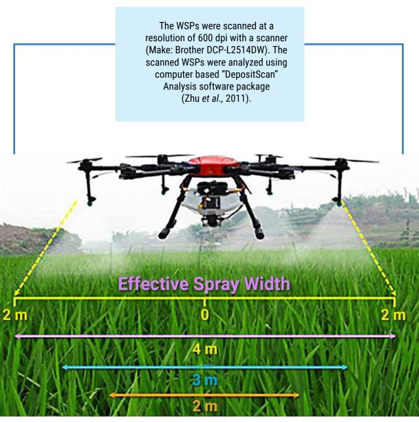
Fig. 6.9 Measuring of spray swath width
