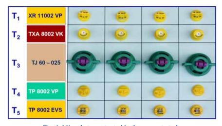
Fig. 6.4 Nozzle types tested in the present study
