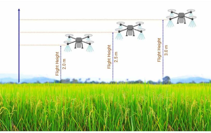
Fig. 6.6 Drone flying test heights
