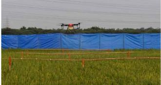
Fig. 6.8 Placement of water sensitive papers at each sampling position for measuring spray swath width
