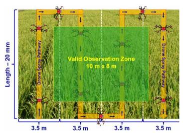
Fig 6.15 Layout of each plot depicting drone path
